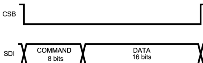
Figure 9. SPI Command and Data Words
