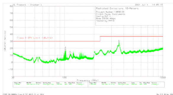
V_{OUT} = 5\text{ V} F_{SW} = 400\text{ kHz} I_{OUT} = 10\text{ A} Frequency Tested: 30 MHz to 1 GHz Figure 9-46. Radiated EMI Bicon Vertical versus CISPR11/32 Limits
