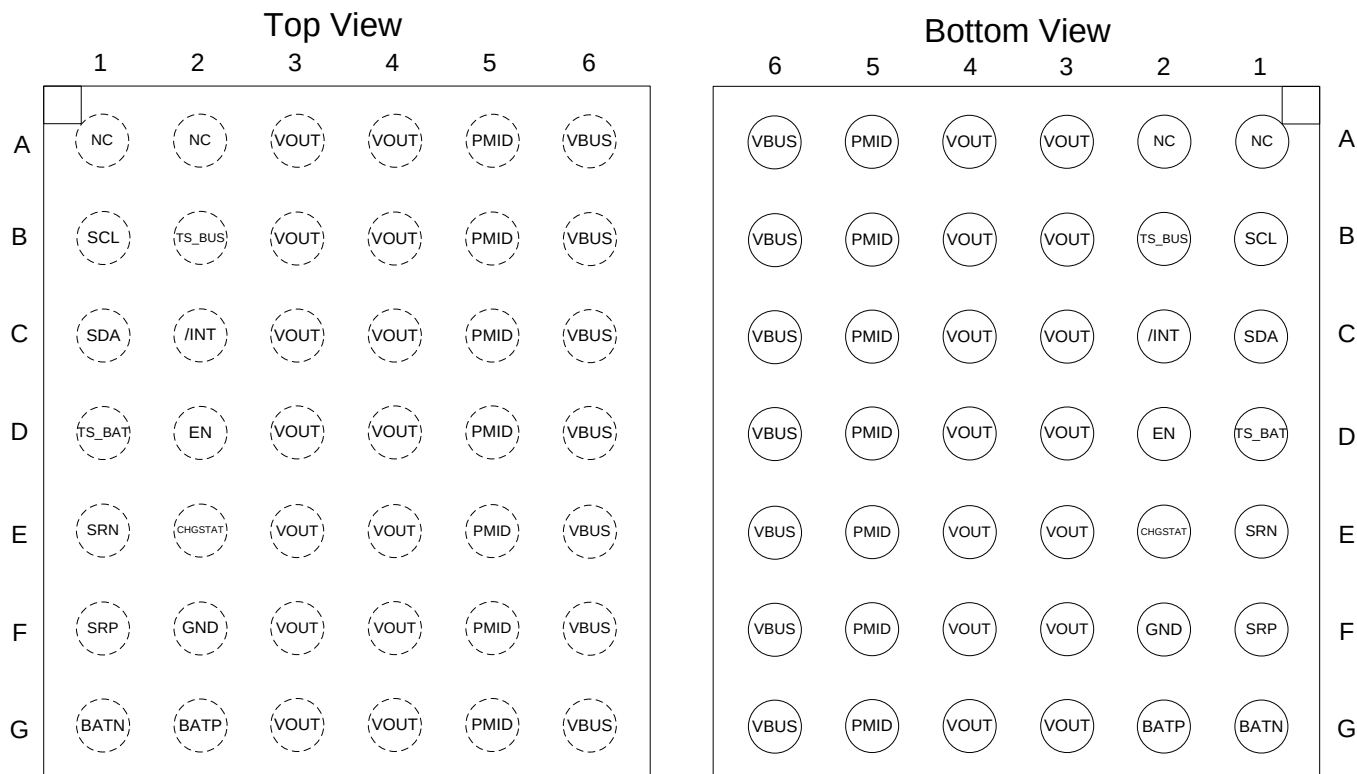
DSBGA Package 42 Pin YYF Top View
