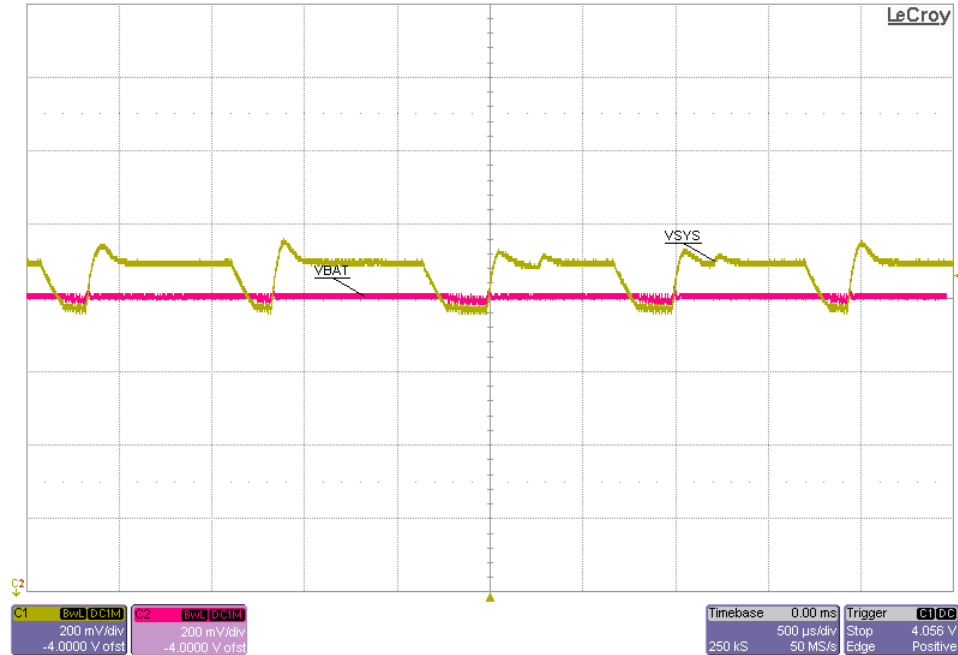
Figure 8-7. V(SYS) When Reverse Boost Prevention Circuit is Active
