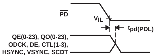
Figure 7. Delay From \overline{\text{PD}} Low to Hi-Z Outputs
