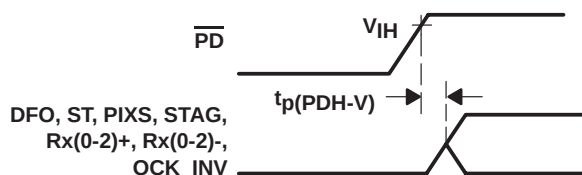
Figure 9. Delay From \overline{\text{PD}} Low to High Before Inputs are Active
