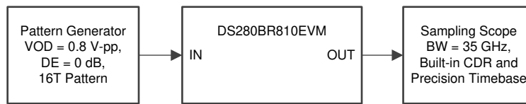
Figure 23. FIR Test Setup
