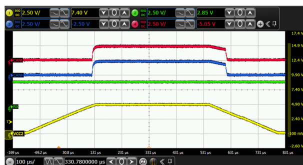
Figure 6-14. Glitch Free Power Up on V_{CC2} – CAN Bus Remains Recessive
