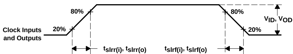
Figure 7. Input and Output Slew Rates
