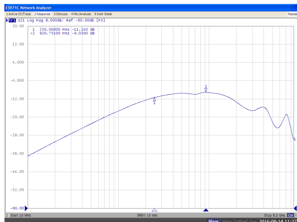
Figure 6-34. Off-State Data-Switch Isolation vs Frequency
