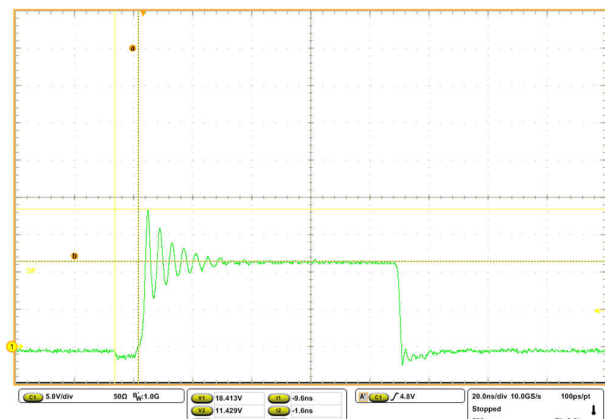
Figure 6-22. Switch Node Ringing and Dead-Time at 10-A Output Current
