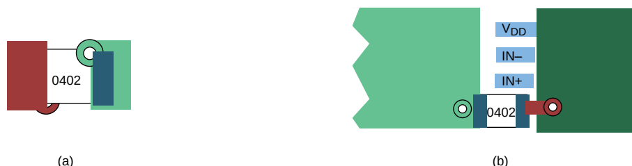
Figure 29. Typical Decoupling Capacitor Layouts
