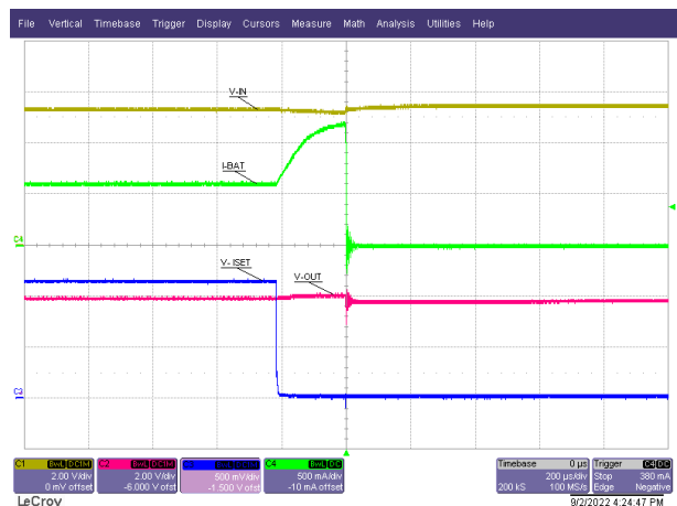
Figure 8-7. OUT Transient Response
