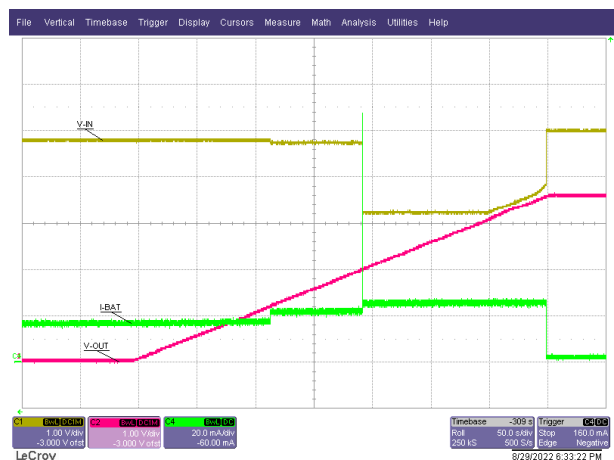
Figure 8-9. ISET Short-Circuit Response
