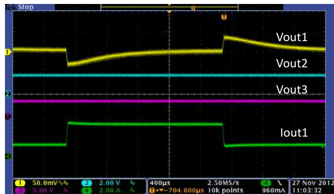
Figure 22. Transient Response Buck1@1.2V, 1-3A Step, C_o = 68\mu\text{F}
