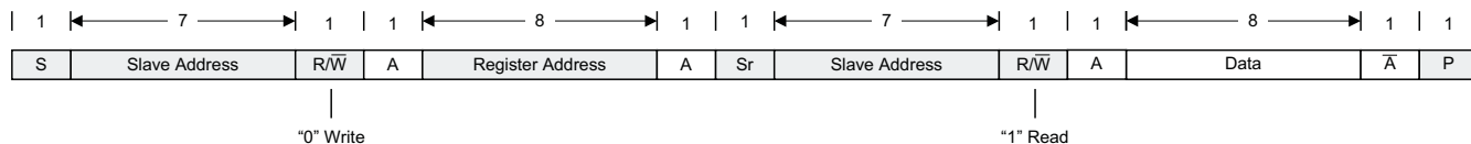
Figure 54. "Write" Data Transfer Format in Standard, Fast- and Fast-Plus Modes
