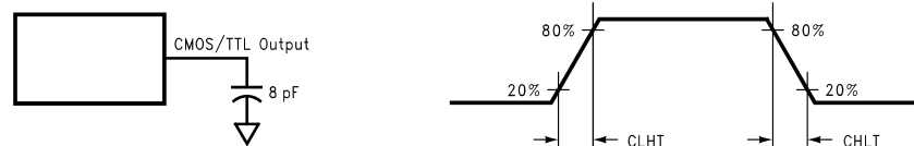
Figure 4. Receiver CMOS/TTL Output Load and Transition Times
