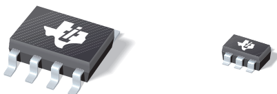
Package Height Comparison (to Scale)
