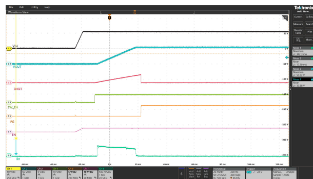
Figure 6-13. Allowed Operating Area (AOA) in Startup
