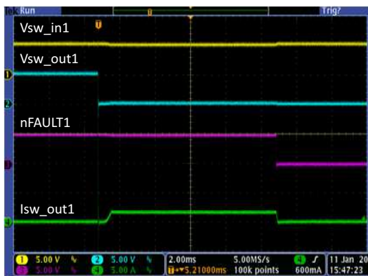
Figure 30. Power Switch1 Current Limit Operation
