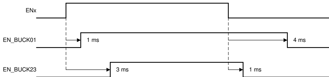
Figure 10. Typical Start-Up and Shutdown Sequencing
