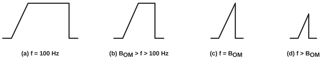
Figure 5. Full-Power-Response Output Signal
