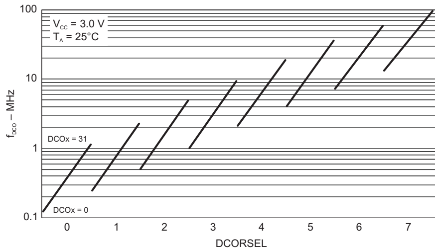
Figure 5-13. Typical DCO Frequency
