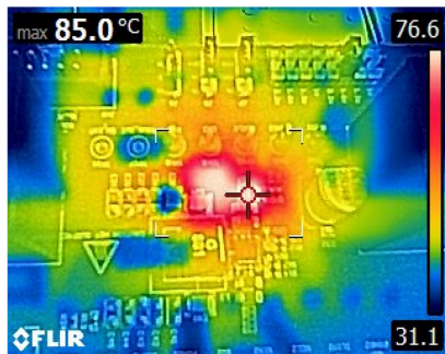
Figure 5-7. Thermal Image – 5V Output, TPS54KB20EVM, 6 Layers
