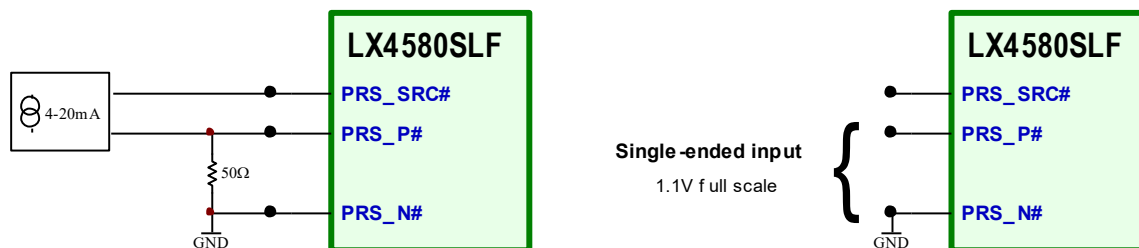
Figure 9. 4-20mA Sensor Connection or General Purpose ADC Connection
