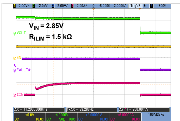
FIGURE 2-3: Overcurrent Fault Response Delay Time.
