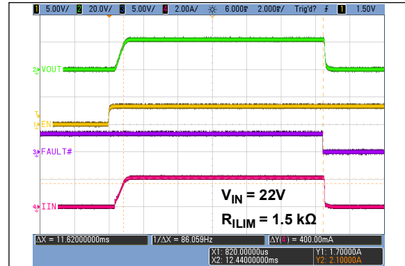
FIGURE 2-4: Overcurrent Fault Response Delay Time.
