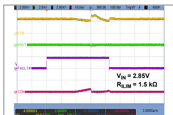
FIGURE 2-18: Turn-On into Short to GND.
