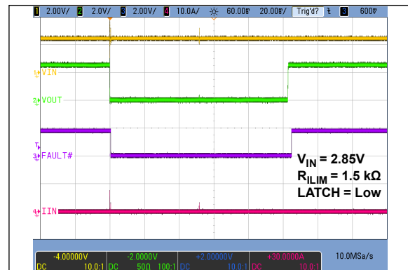
FIGURE 2-16: Output Recovery from Short Circuit.
