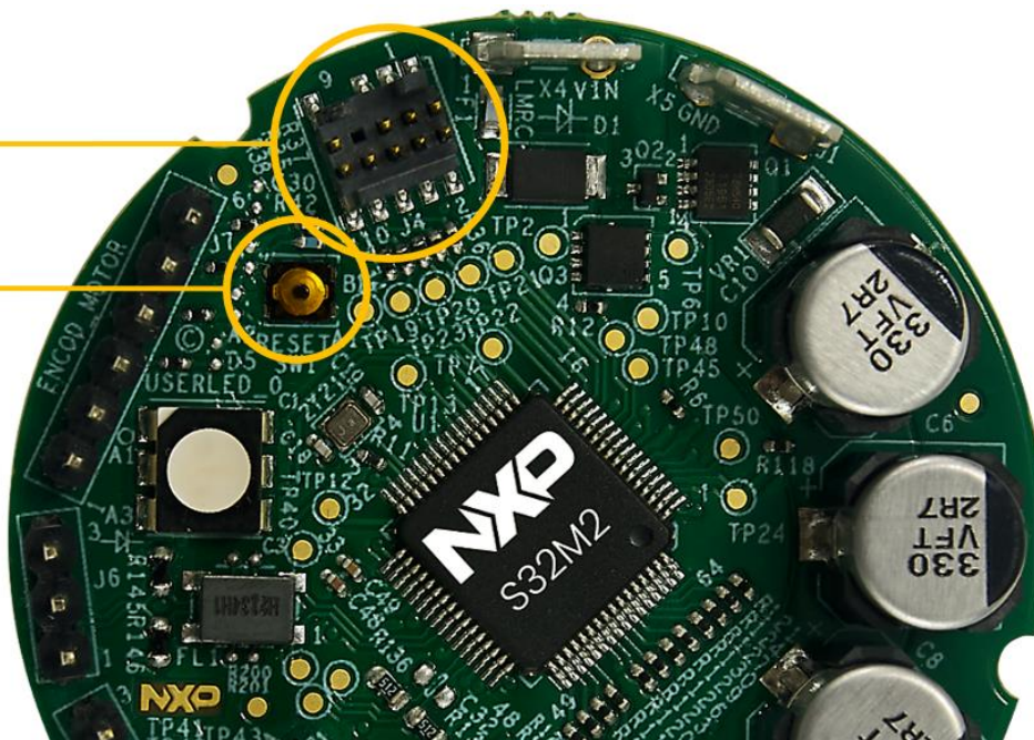
Figure 11. S32M276SFFRD – JTAG connector and RESET Switch
