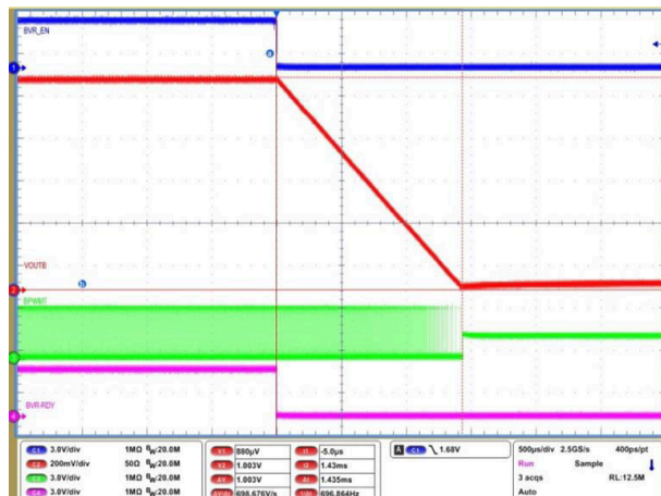
Figure 8-20. Soft-stop channel B (0 ms TOFF_DELAY)
